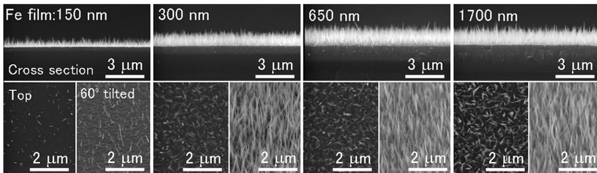
Fig. 2. SEM images of α-Fe<sub>2</sub>O<sub>3</sub> nanowires synthesized from Fe films with thicknesses of 150, 300, 650 and 1700 nm. The annealing time was 30 min. Upper panels show cross-sectional images. Lower panels show top-view and tilted (60°) images.
