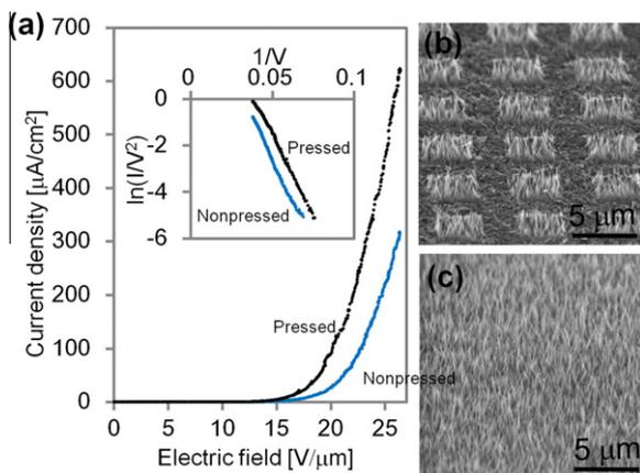
Fig. 6. (a) Current density versus electric field ( $I$ - $V$ ) plots for  $\alpha$ -Fe<sub>2</sub>O<sub>3</sub> nanowires patterned by pressing and nonpressed  $\alpha$ -Fe<sub>2</sub>O<sub>3</sub> nanowires. The inset shows their Fowler-Nordheim ( $F$ - $N$ ) plots. (b) A SEM image of nanowires patterned by press (tilt angle: 60°). (c) A SEM image of as non-pressed nanowires (tilt angle: 60°).
