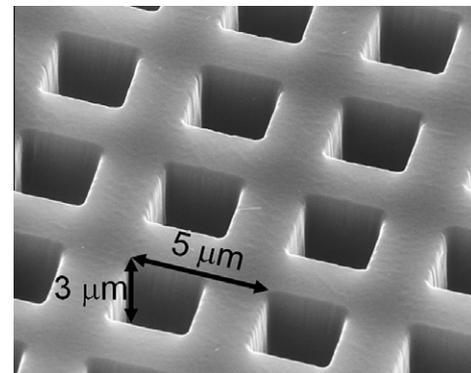
Fig. 4. SEM image of microstructured mold (tilt angle: 40°).
