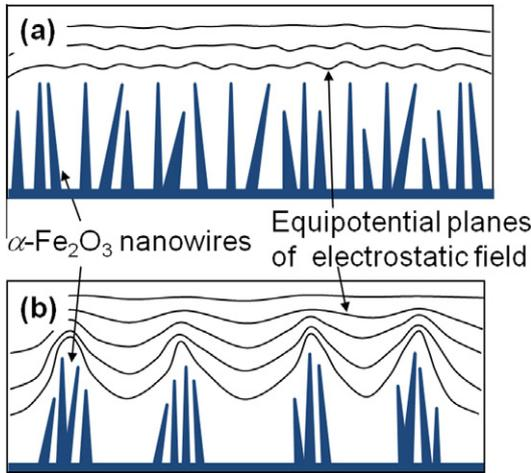
Fig. 1. Schematics of electric fields around (a) uniformly and (b) discretely synthesized nanowires.
