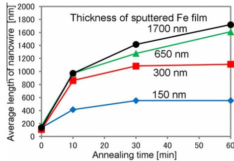
Fig. 3. Average lengths of α-Fe<sub>2</sub>O<sub>3</sub> nanowires synthesized from Fe films with thicknesses of 150, 300, 650 and 1700 nm with annealing times of 0, 10, 30 and 60 min.
