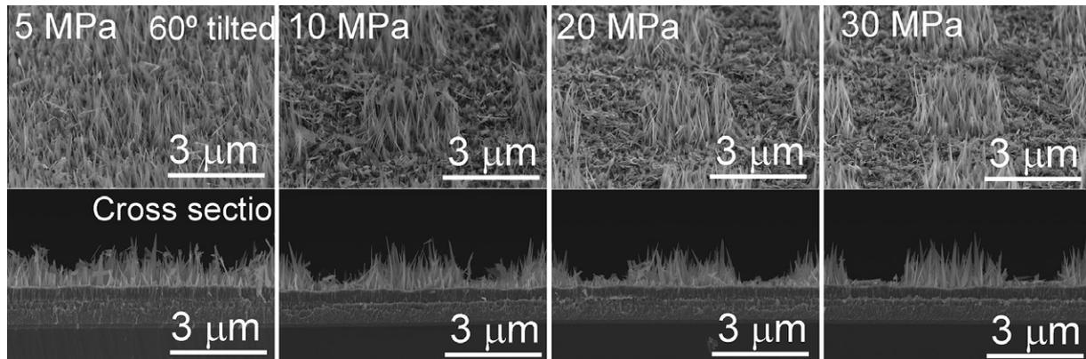
Fig. 5. SEM images of patterned  $\alpha$ -Fe<sub>2</sub>O<sub>3</sub> nanowires pressed at 5, 10, 20 and 30 MPa. Upper panels show tilted (60°) images and lower panels show cross-sectional images.
