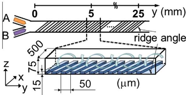
Fig. 1. Schematic of our slurry mixing device.
