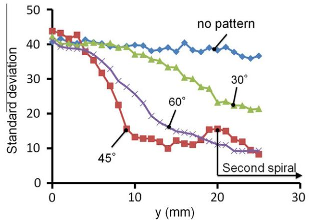
Fig. 3. Plots of the standard deviation of intensity distribution in microscopy images in Fig. 2. as a function of the distance along the channel,  $y$ .
