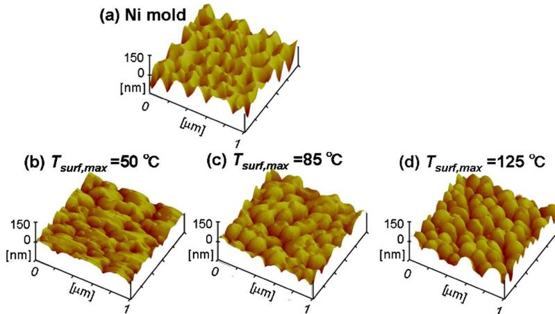
FIG. 5. (Color online) AFM profiles of (a) Ni mold and imprinted PS in injection molding, with the peak temperatures of the mold surface of (b) 50, (c) 85, and (d) 125 °C.
