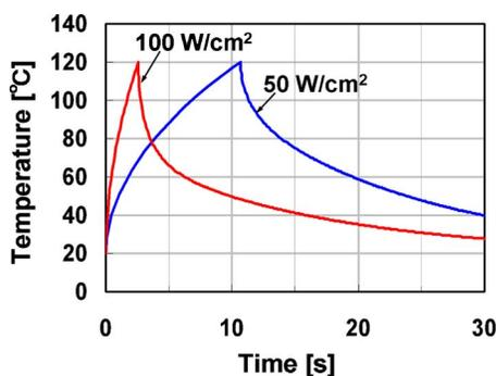
FIG. 2. (Color online) Finite element method simulation results of rapid heating and cooling.
