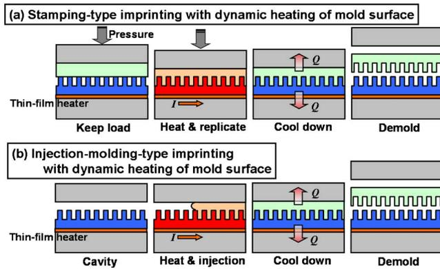
FIG. 1. (Color online) Schematics of rapid thermal imprinting by dynamic heating of mold surface: (a) stamping method and (b) injection molding method.
