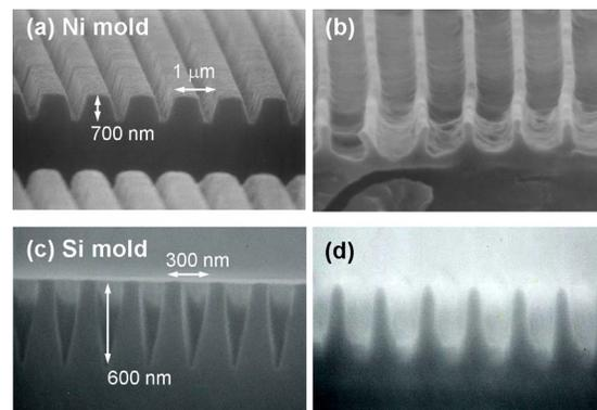
FIG. 4. (Color online) Cross-sectional SEM images of nanostructured mold and imprinted PMMA in stamping-type imprinting: (a) Ni mold, (b) imprinted PMMA using (a), (c) Si mold, and (d) imprinted PMMA using (c).
