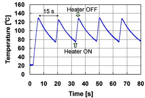
FIG. 3. (Color online) Result of cyclic test of heating/cooling. The heater is turned off when the mold surface temperature reaches 130 °C, and turned on when it reaches 75 °C.
