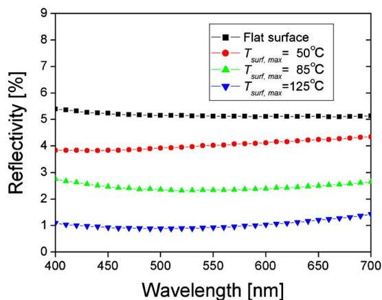
FIG. 6. (Color online) Reflectivities of flat PS surface imprinted at 50, 85, and 125 °C.
