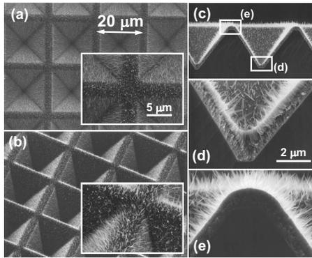
FIG. 5. SEM images of nanowires synthesized from a patterned substrate (20  $\mu\text{m}$  pitch pyramidal holes). (a) Top images, (b) tilted images (45°), and [(c)–(e)] cross-section images. The annealing time was 30 min.
