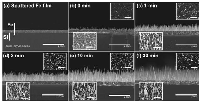
FIG. 1. Cross-sectional SEM images of the Fe thin film (a) and synthesized iron oxide nanowires with annealing times of 0 (b), 1 (c), 3 (d), 10 (e), and 30 min (f). The insets show top and tilted images ( $45^\circ$ ). All the scale bars indicate  $2 \mu\text{m}$ .
