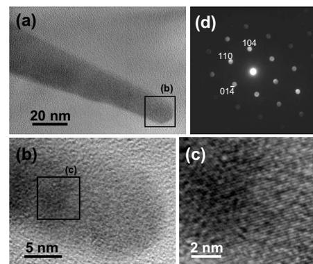
FIG. 4. TEM images of a nanowire. (a) Low-magnification image, [(b) and (c)] high-magnification images, and (d) diffraction pattern.
