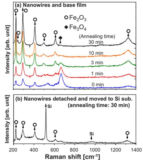
FIG. 3. (Color online) Raman spectra of (a) the nanowire substrates annealed for 0/1/3/10/30 min and (b) nanowires which was removed from the substrate onto a Si substrate.
