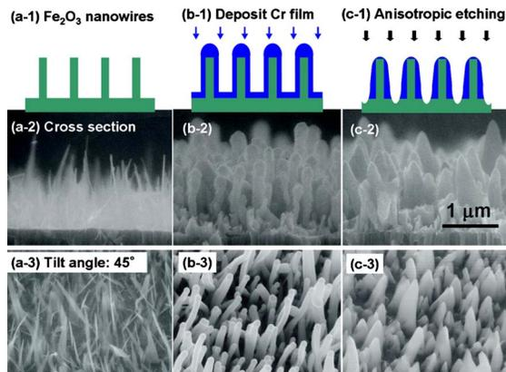
FIG. 2. (Color online) Schematic of fabrication of array of conical structures; nanowire synthesis (a)(1), Cr deposition (a)(2), and anisotropic  $\text{CHF}_3$  etching (a)(3). Cross-sectional SEM images [(b)(1)–(b)(3)] and 45°-tilted views [(c)(1)–(c)(3)] at each step.
