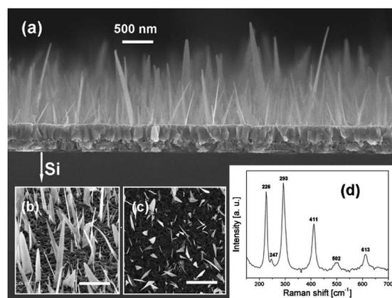
FIG. 1. Iron oxide nanowires synthesized from sputtered thin Fe film. SEM image of cross section (a), 45°-tilted view (b), top view (c), and Raman spectrum of the nanowire substrate (d).
