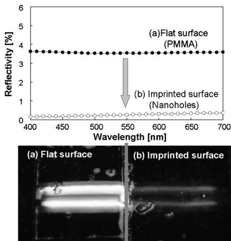
FIG. 5. Reflectivities and optical images of PMMA flat surface (a) and imprinted surface (b). The films were attached on a black PMMA plate using an optically matched tape and an image of fluorescent light reflected from each film was obtained.
