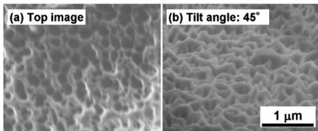
FIG. 4. SEM images of imprinted PMMA film; cross section (a) and tilted view (b).
