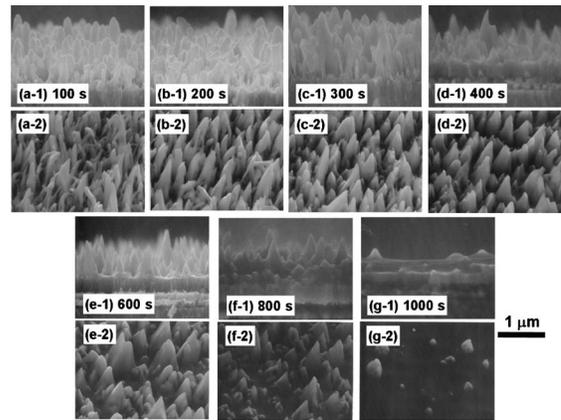
FIG. 3. SEM images of array of conical structures after various etching times (100/200/300/400/600/800/1000 s).
