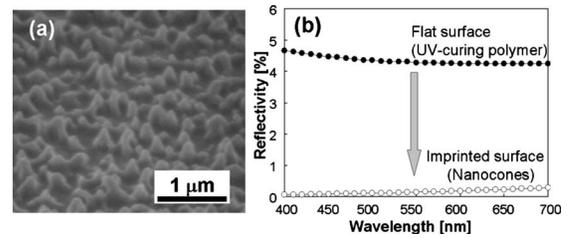
FIG. 6. UV-curable polymer imprinted using the PMMA replica mold (Fig. 5). SEM image taken from 45° (a) and reflectivities of flat and imprinted surfaces (b).
