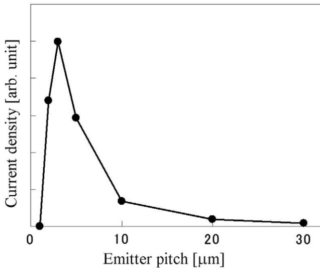
Fig. 6. Simulation results of current density as a function of emitter pitch.
