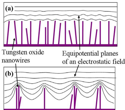
Fig. 1. Schematics of electric fields around (a) uniformly- and (b) discretely-synthesized tungsten oxide nanowires.
