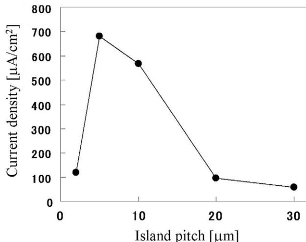
Fig. 4. Current density at electric field of 38  $\text{V}/\mu\text{m}$  plotted as a function of island pitch.
