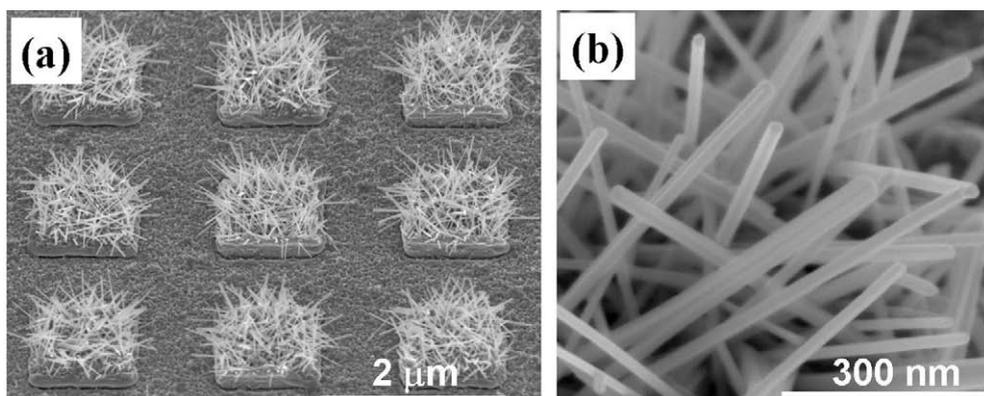
Fig. 2. (a) SEM image of tungsten oxide nanowires synthesized on islands (Tilt angle: 45°). (b) Enlarged SEM image of tungsten oxide nanowires.
