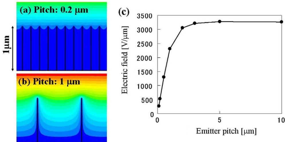
Fig. 5. (Color online) Simulation results of electric field profiles: (a) 0.2  $\mu\text{m}$  pitch, (b) 1  $\mu\text{m}$  pitch. (c) Electric field at the tip of emitters as a function of emitter pitch.
