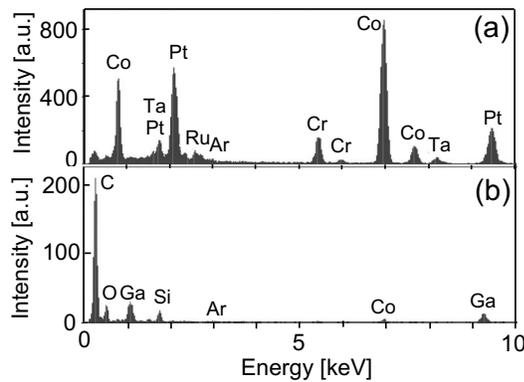
FIG. 5. EDS of (a) amorphous carbon and (b) magnetic layer after Ar-GCIB irradiation with an ion dose of  $5 \times 10^{14}$  ions/cm<sup>2</sup>.
