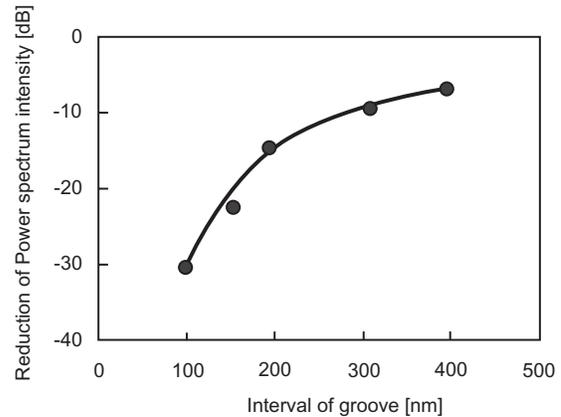
FIG. 4. Dependence of the reduction in carbon roughness power spectral intensity on groove interval.
