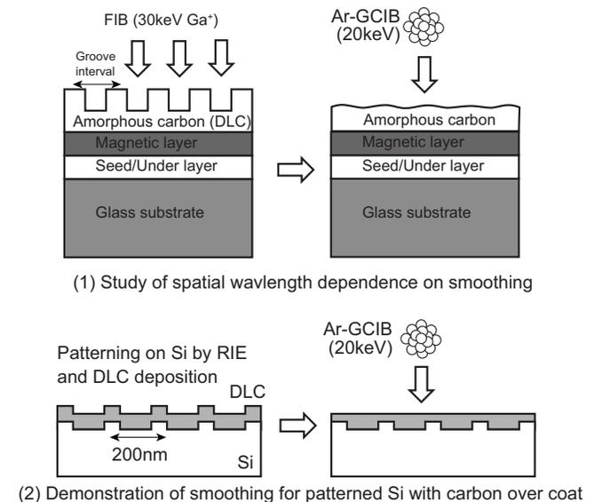
FIG. 1. Experimental procedures.
