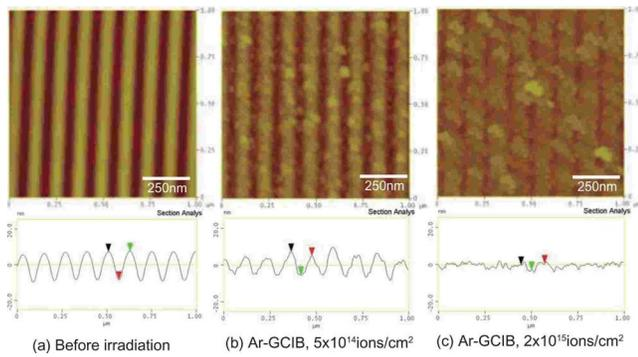
FIG. 2. (Color online) Surface morphology and cross-section profile of AFM before and after Ar-GCIB irradiation with acceleration energy of 20 keV. The ion doses were (b)  $5 \times 10^{14}$  ions/cm<sup>2</sup> and (c)  $2 \times 10^{15}$  ions/cm<sup>2</sup>.
