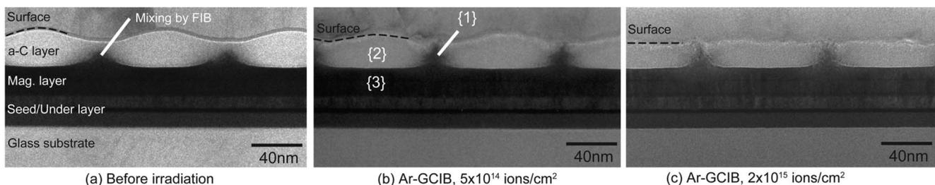
FIG. 3. Cross-sectional TEM view of grooves on amorphous carbon after irradiation of Ar-GCIB (acceleration energy: 20 keV; ion dose:  $5 \times 10^{14}$  and  $2 \times 10^{15}$  ions/cm<sup>2</sup>).
