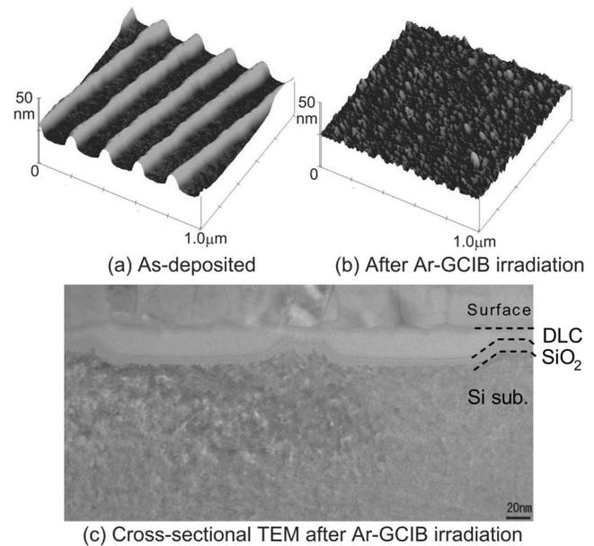
FIG. 6. Cross-sectional TEM image of the patterned Si with carbon overcoat after Ar-GCIB irradiation (acceleration voltage=20 kV; ion dose= $2 \times 10^{15}$  ions/cm<sup>2</sup>). AFM images of before and after Ar-GCIB irradiation are also presented.
