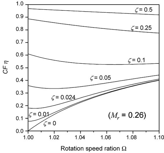
Fig. 4. Analytical CF as a function of rotation speed ratio ( $\Omega$ ), when  $M_r = 0.26$  (experimental value in this study) and  $\zeta = 0, 0.01, 0.024, 0.05, 0.1, 0.25,$  and  $0.5$ .
