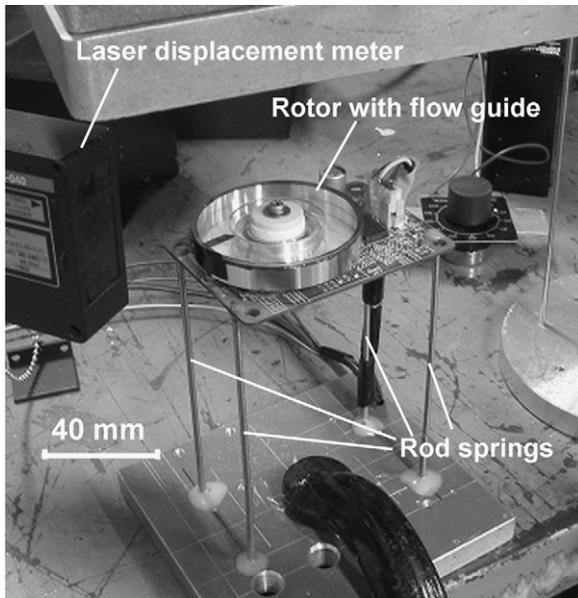
Fig. 7. Experimental setting for automatic unbalance correction system using UV-curing resin.
