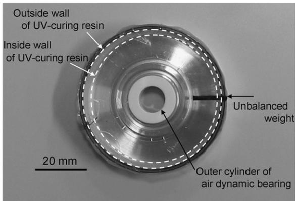
Fig. 10. Rotor corrected by UV-curing resin.
