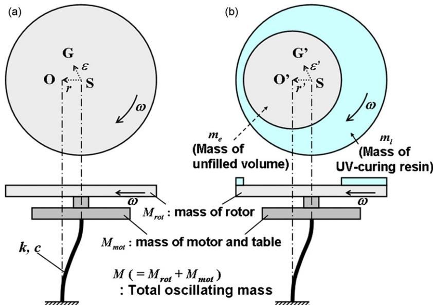
Fig. 3. Oscillation models (a) without and (b) with UV-curing resin.
