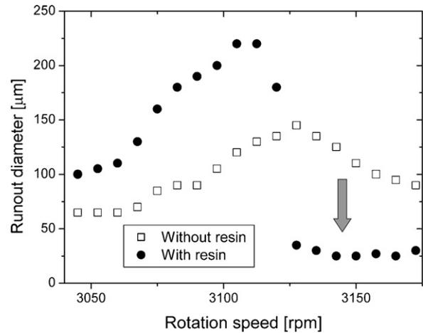
Fig. 8. Experimental result of the runout diameter as a function of rotation speed, with and without UV-curing resin.
