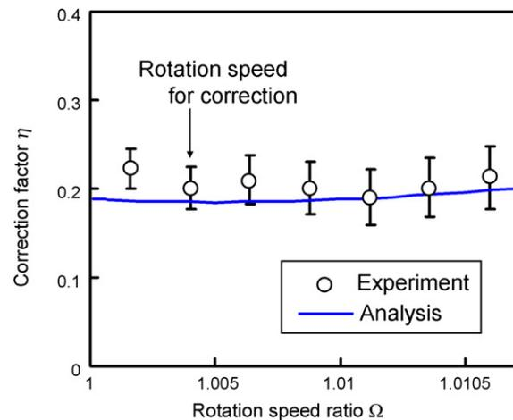
Fig. 9. Correction factor as a function of  $\Omega$  obtained by experiment and analysis.
