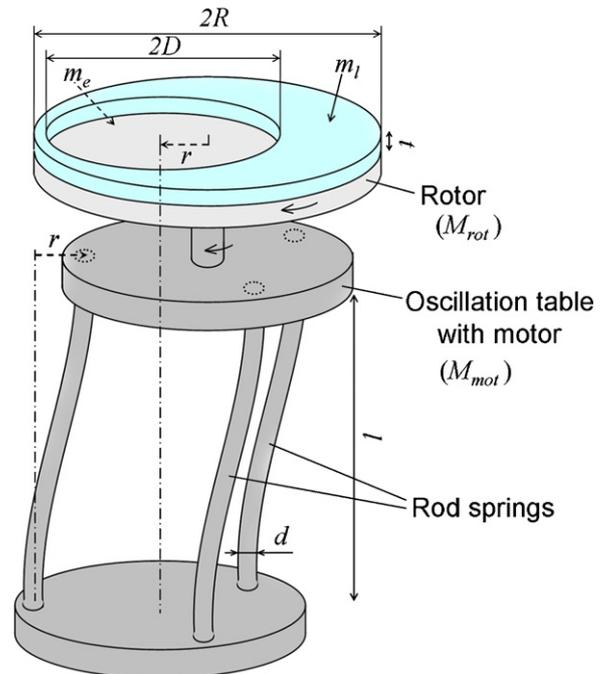
Fig. 6. Design parameters of flow guide for UV-curing resin and translational oscillation system.
