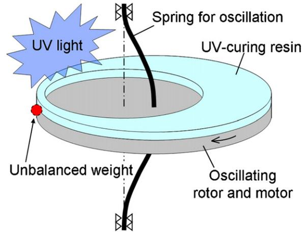
Fig. 2. Schematic of automatic unbalance correction using UV-curing resin.
