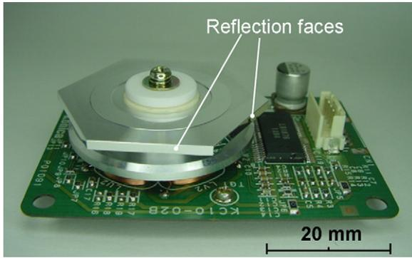
Fig. 1. Polygon scanner motor by Konica Minolta Business Technologies, Ltd. (regular rotation speed: 20,000–60,000 rpm).
