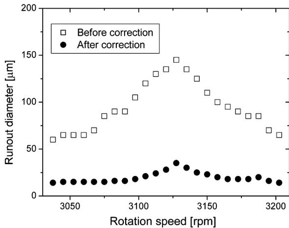
Fig. 11. Runout diameter before and after automatic unbalance correction.
