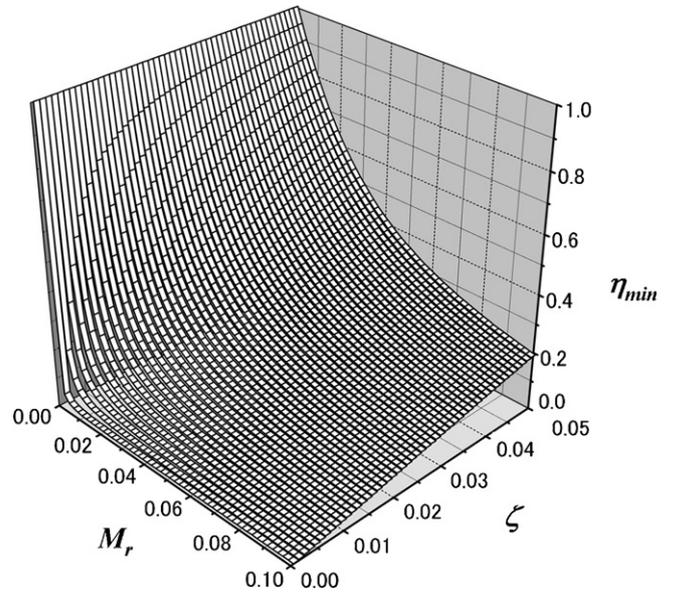
Fig. 5. Analytical minimum correction factor ( $\eta_{min}$ ) as function of mass ratio ( $M_r$ ) and damping ratio ( $\zeta$ ).
