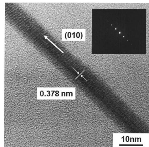
FIG. 6. TEM image of a synthesized nanowire.
