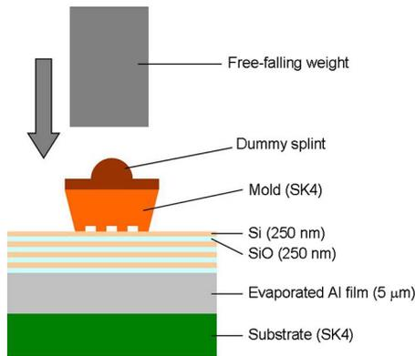
FIG. 2. Schematic of experimental setup for testing high-speed shearing of multilayer thin films.
