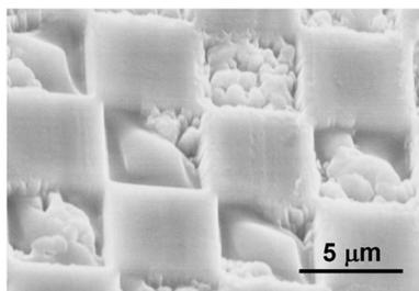
FIG. 3. SEM image of checker-patterned mold fabricated by FIB (tilt angle:  $40^\circ$ ).
