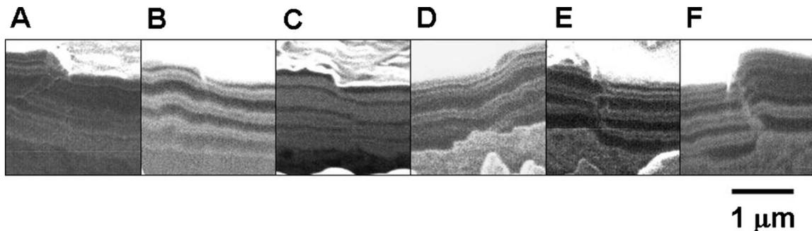
Fig. 6. SIM images of cross sections of deformed layer under conditions listed in Table I (A–F). Tilt angle:  $60^\circ$ .
