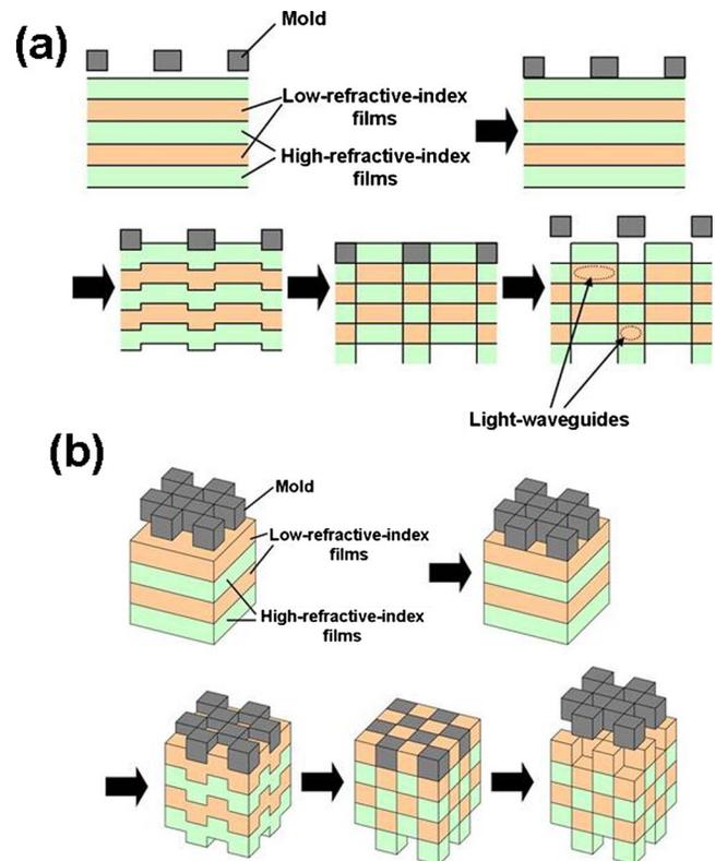
FIG. 1. Schematic of single-pass forming of (a) chip-based light waveguides and (b) 3D periodic microstructures using high-speed shearing of multilayer thin films.
