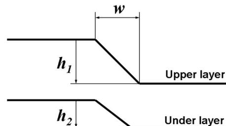
FIG. 5. Deformation model for determining strain.
