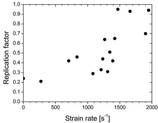
FIG. 7. Replication factor as a function of strain rate.
