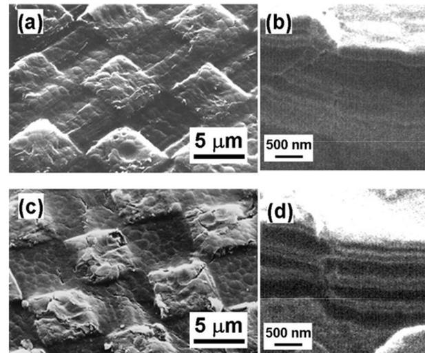
FIG. 4. (a) SEM surface image (tilt angle:  $40^\circ$ ), (b) SIM cross-sectional image (tilt angle:  $60^\circ$ ) of sample pressed statically (mass of weight: 4.3 kg), (c) SEM surface image, and (d) SIM cross-sectional image of sample pressed at high strain rate (mass of weight: 75 g, strain rate:  $1500\ \text{s}^{-1}$ ).
