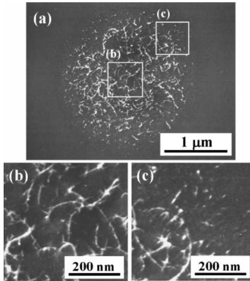
Fig. 3. SEM images of SWNTs synthesized by laser-assisted CVD for laser-irradiation time of 1 s: (a) entire circular area, (b) center and (c) edge of area.
