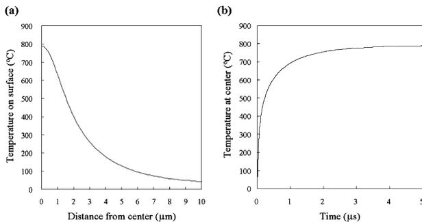
Fig. 6. (a) Calculated temperature distribution on surface of multilayer substrate. (b) Calculated time variation of temperature at center of surface.
