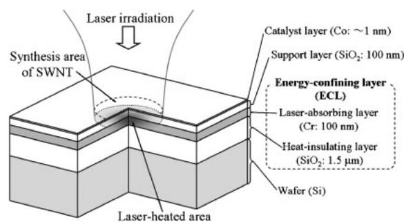
Fig. 1. Schematic of laser-assisted CVD synthesis of SWNTs on multilayer substrate with ECL.
