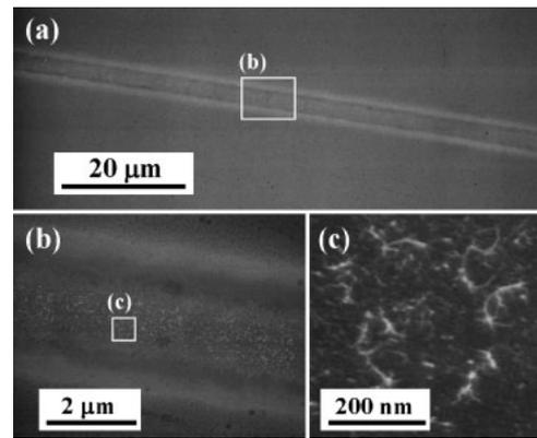
Fig. 7. SEM images of line-patterned synthesis of SWNTs by scanning of laser-irradiation spot: (a) entire region, (b) enhanced area, and (c) highly magnified image of enhanced area.
