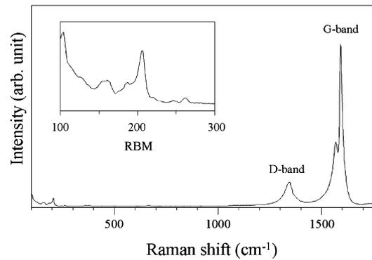
Fig. 4. Raman spectra of synthesized SWNTs. The excitation wavelength was 488 nm at a spot diameter of 4  $\mu\text{m}$ .
