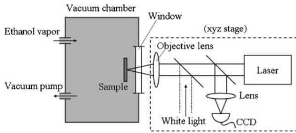
Fig. 2. Configuration of experimental apparatus for laser-assisted CVD synthesis of SWNTs.
