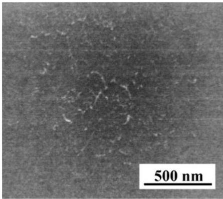
Fig. 5. SEM image of localized synthesis of SWNTs in area of about 1  $\mu\text{m}$  diameter.
